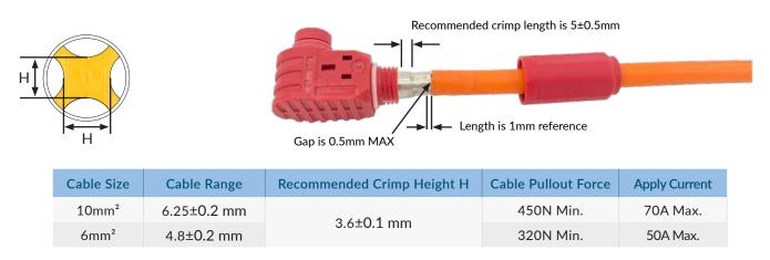
Notes: The recommended crimp sizes are only for reference. The customer should adjust them according to cable specification and crimp tool. Test results including temperature rise, metallographic analysis, and pullout force. Recommended crimping tool: Hydraulic press
